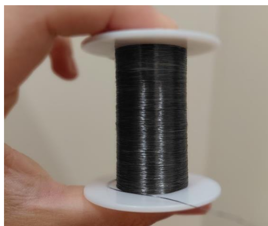
Carbon Nanotube Molecular Structure Wound into yarn (CNTy)
