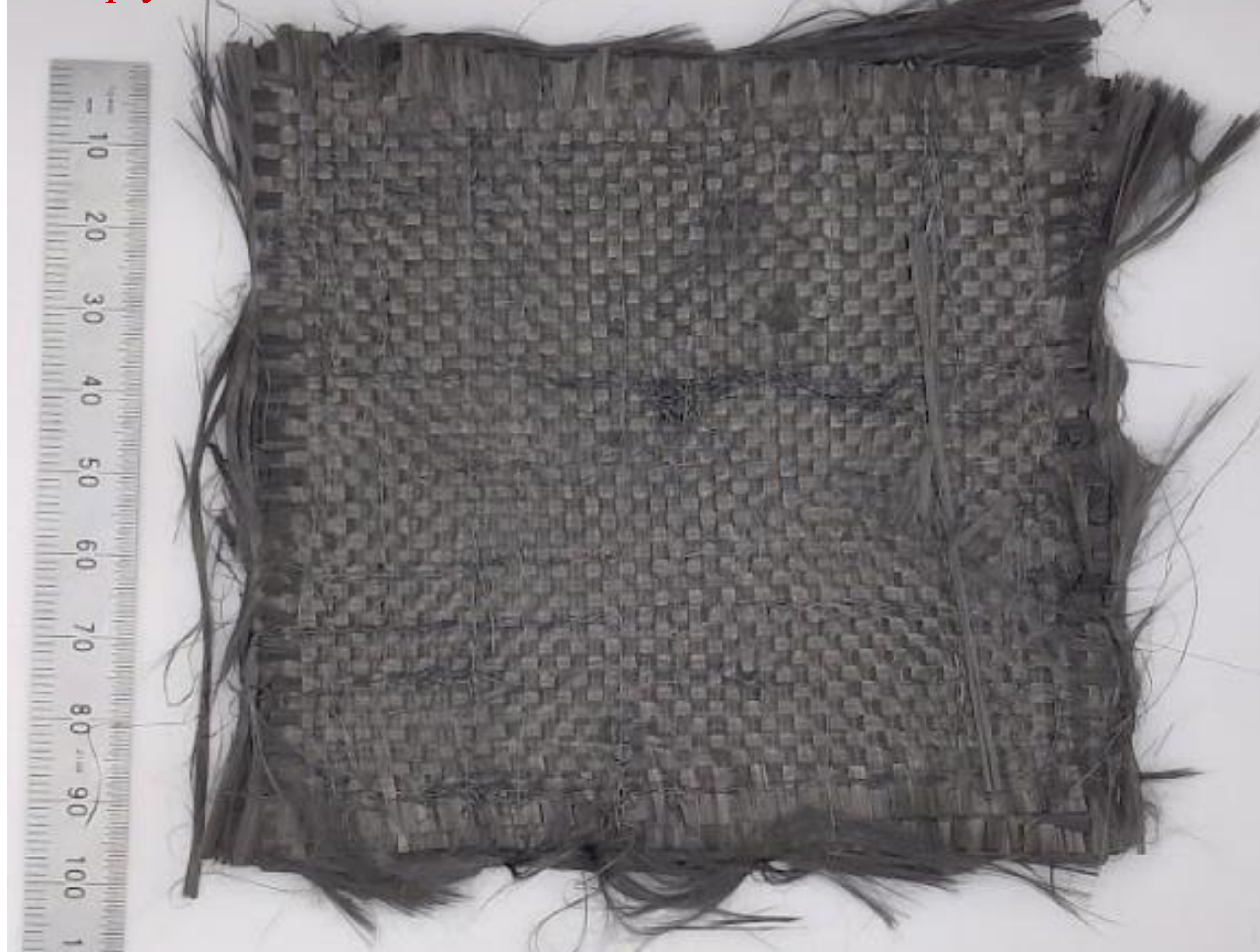
12-ply IM7 Carbon Fiber Z-stitched
